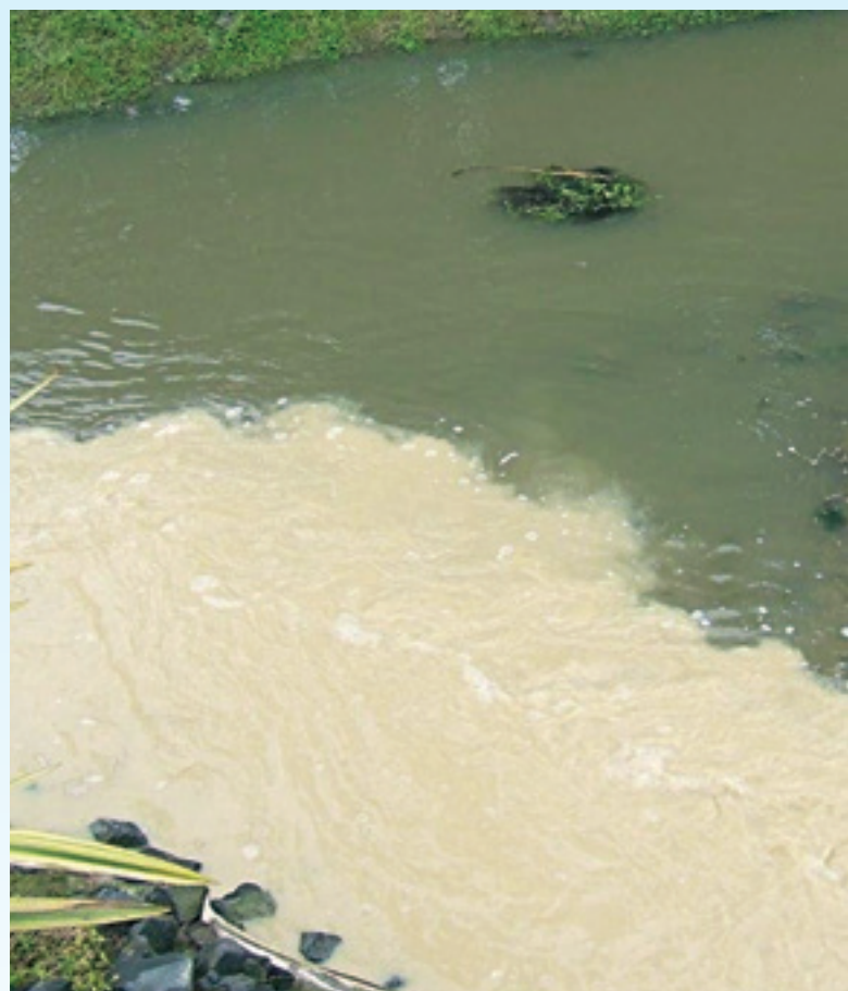
Both these photos show unacceptable sediment levels in the river. In the photo on the left sediment is contaminating clear water. On the right, poor water is being further contaminated. Both show a conspicuous change in water colour, therefore, they fail the sediment runoff rule.
