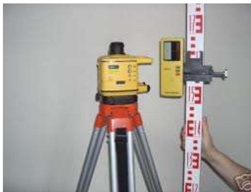
Figure 4 – Example of a laser level and sensor
