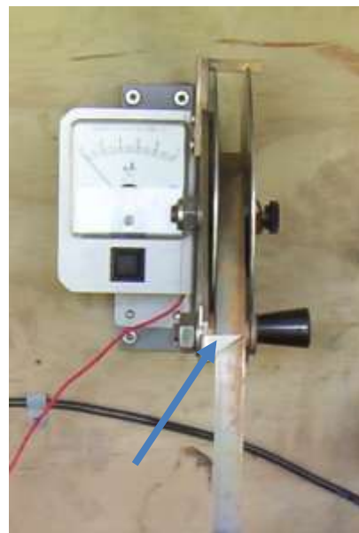
Figure 26 – Electric plumb bob with electric pointer as the reference
