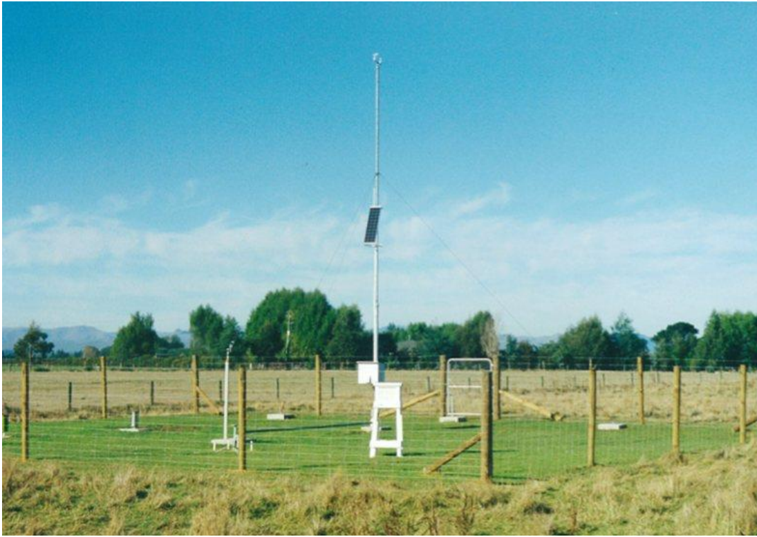
Figure 5 – Example of a 10-m tilting mast
