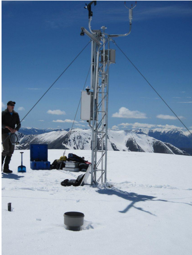
Figure 7– Example of a 3-m lattice mast Photo: Courtesy of Andrew Harper, NIWA.
