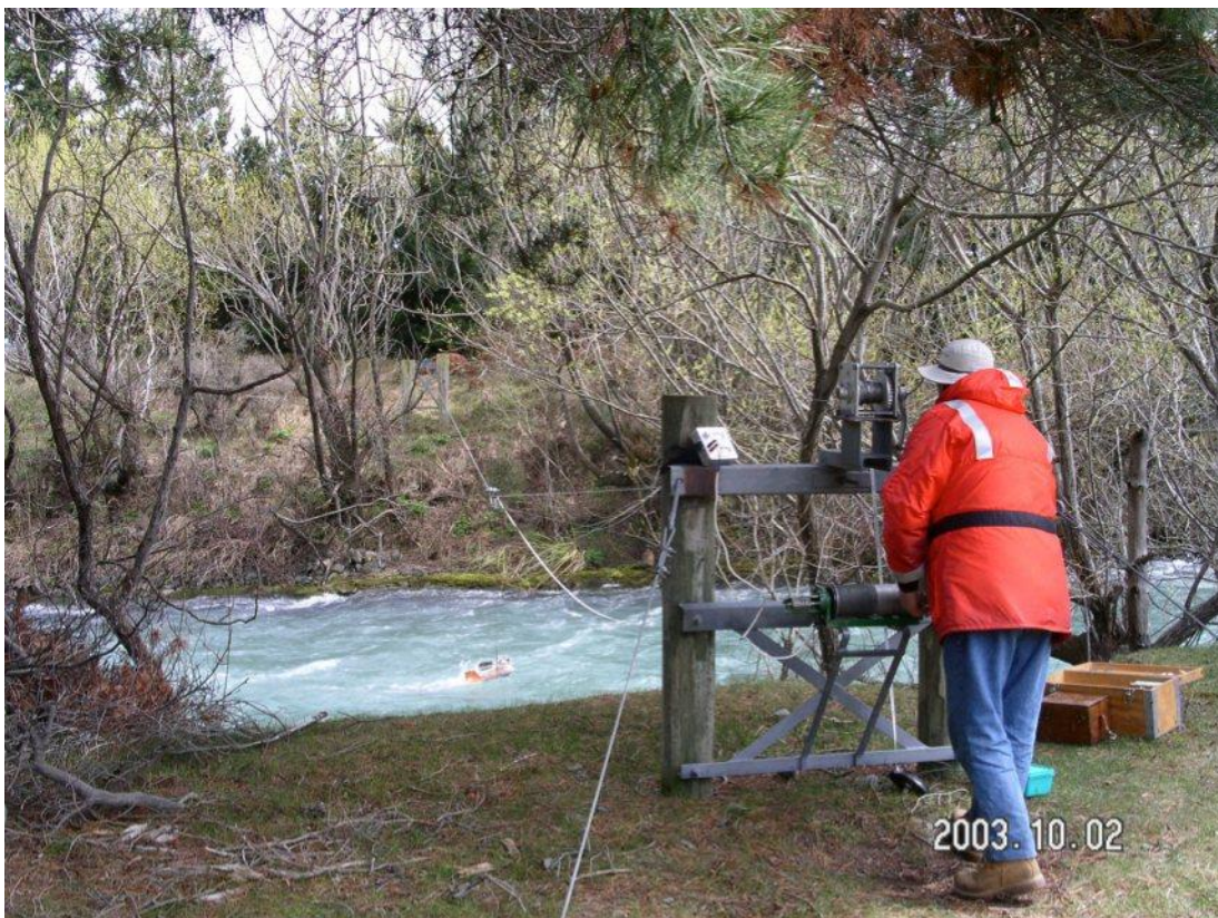
Figure 3 – Flow gauging from a manual winch slack-line cableway
