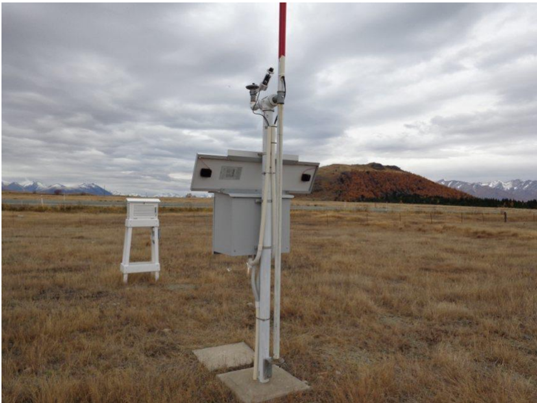
Figure 6 – Example of a 6-m tilting mast
