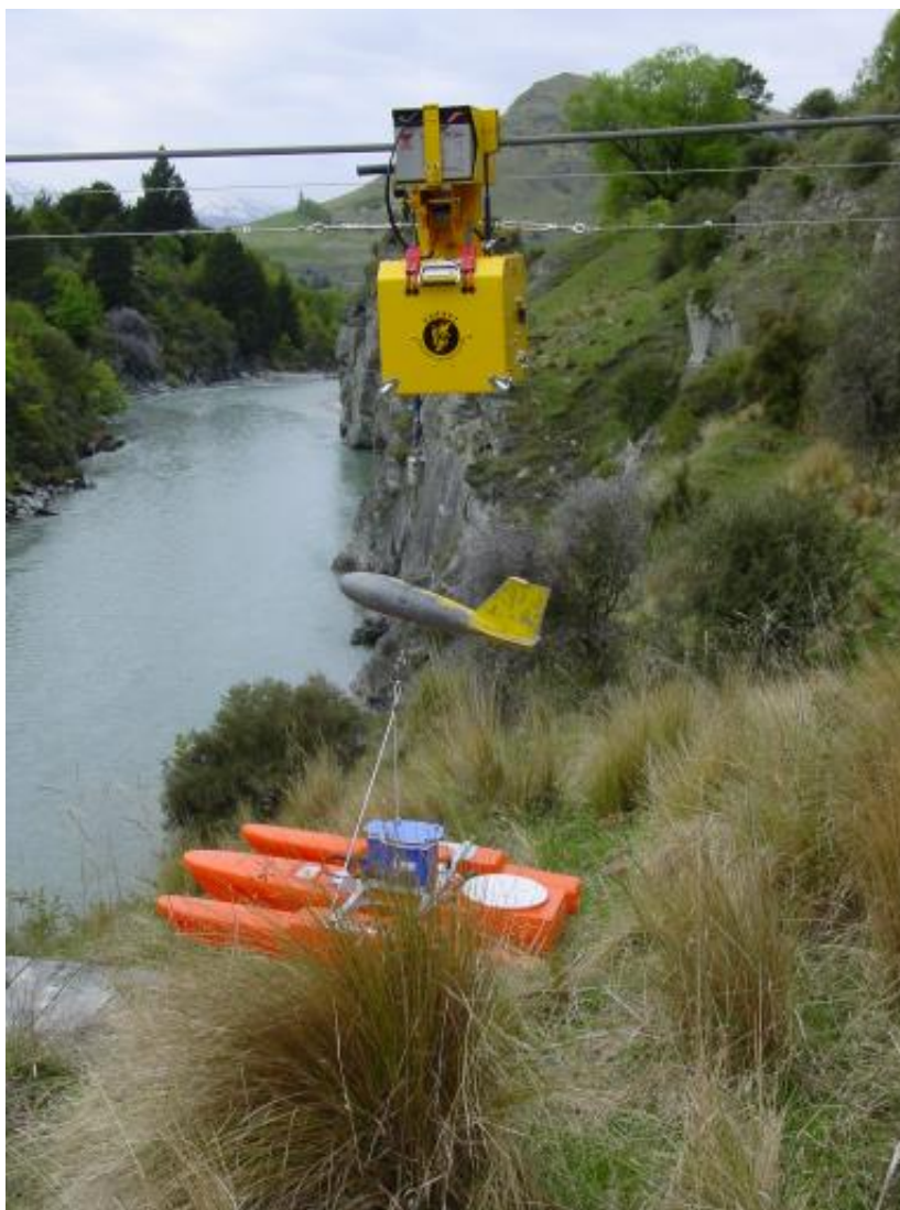
Figure 4 – Flow gauging using a ‘Hornet’ motorised slack-line system retrofitted to a manned cableway
