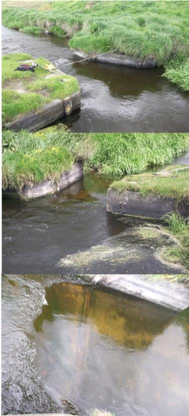
Figure 14 – Awanui Stream Flume Operating Semi-Submerged in the Top and Centre Images, and Under Free-Flow with Formation of a Hydraulic Jump in the Bottom Image
