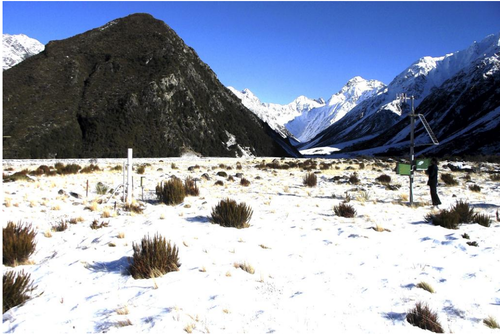
Figure 5 – Primary Reference Gauge 1000 mm above Ground
